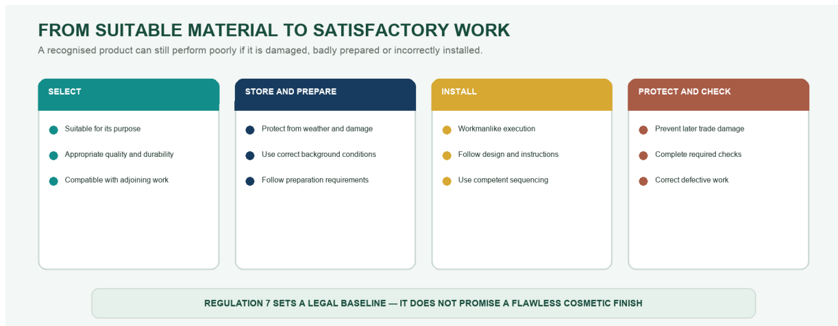
Figure 2. Regulation 7 connects suitable products and materials with appropriate preparation, installation and protection.
