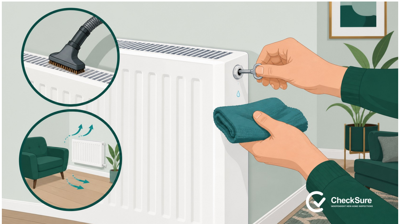
Figure 1. Bleed only a suitable cool wet radiator, using the top-corner valve; keep the radiator clean and airflow unobstructed.
