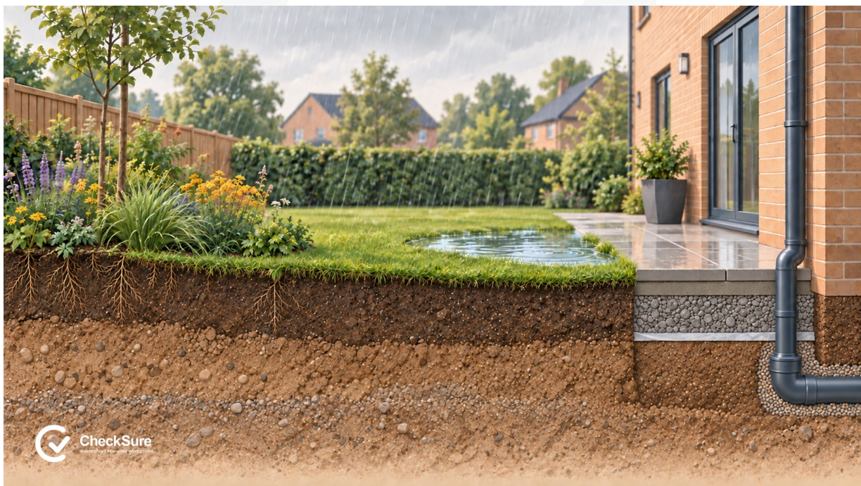
Figure 1. Turf, paving and drainage depend on suitable ground preparation and correctly formed layers below the finished surface.
